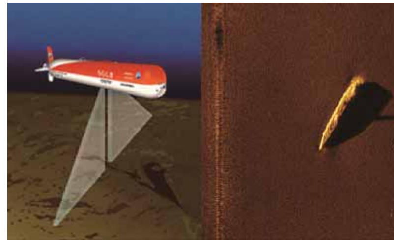
The drawing on the left shows debris mapping using a side scan sonar. The picture on the right shows debris on the bottom of the sea carried by the tsunami. (© JAMSTEC)
