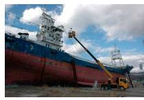
A vessel scanned by a 3D laser scanner
