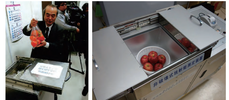
丸ごと汚染検査器の開発 Development of non-destructive radioactive contamination monitoring of food "as a whole".
