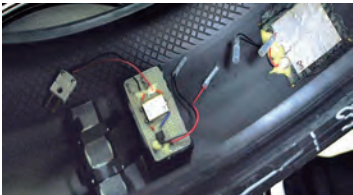
タイヤ内に装着した圧電シートと高蓄電効率電子回路 Car tires equipped with the power generation sheet and high efficiency storage circuits.
